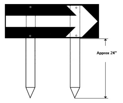
A Direction Marker consists of a 10mm thick Board 4 feet by  $1\frac{1}{2}$  feet with a PVC printed fluorescent yellow arrow on a black background with 2 wooden legs/uprights measuring 2 inches x  $1\frac{1}{2}$  inches x 42 inches as attachments.
